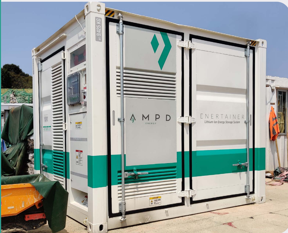
Ampd Energy's "Enertainer" battery system in action on a Hong Kong construction site. (Ampd Energy)
