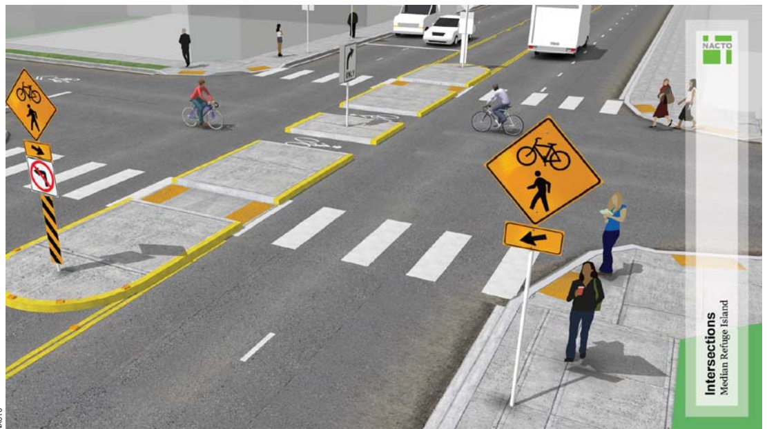
This example from NACTO's Urban Bikeway Design Guide illustrates how a cyclist crossing can be clearly marked on a high-volume road.
