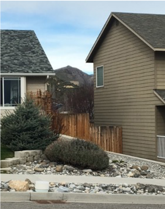
Landscape features like wood mulch, wood fences that connect to structures, and highly flammable plants like juniper bushes should be reduced to limit fire risk in communities.
