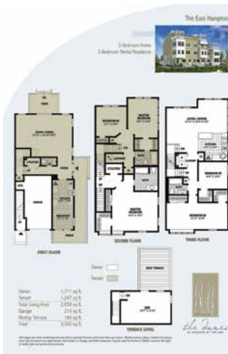
The floor plan for the East Hampton unit in the Dunes. The owner's unit is on the second and third levels, and the rental unit is on the first and second levels.
