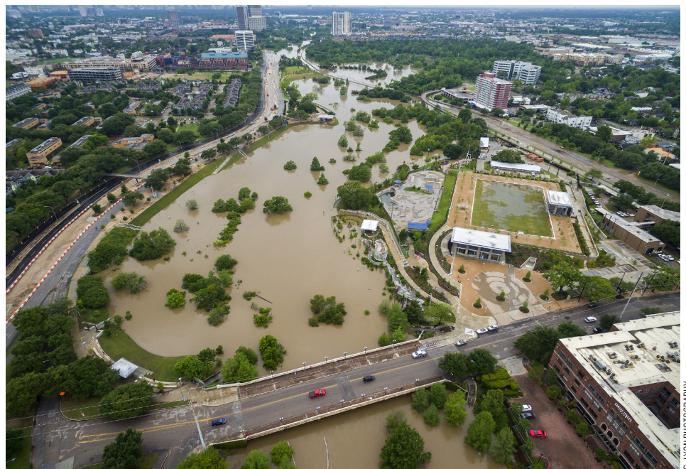
Because the park is built in a floodway, water will rise up to 20 feet several times a year during Houston's sporadic torrential rainfalls, inundating and submerging everything in the park. At the right is the Water Works.
