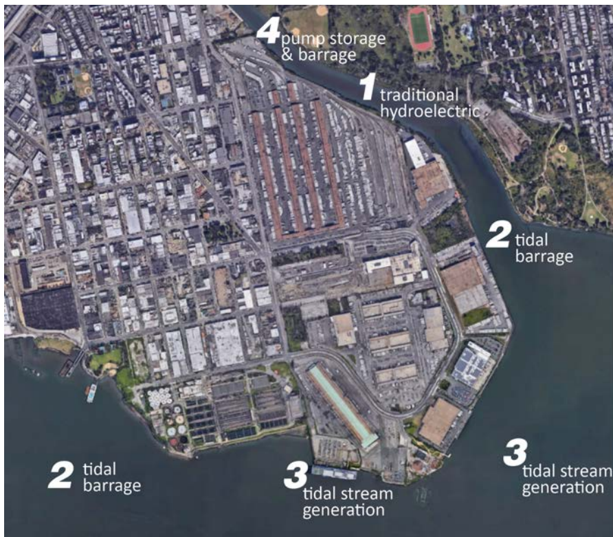
Potential siting of various hydropower installation options at Hunts Point. Source: TAP Panel.
