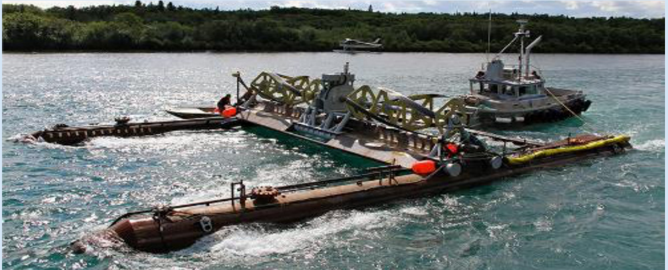
ORPC's RivGen system which as recently been deployed in the remote Alaskan village of Igiugig. Source: Ocean Renewable Power Company.
