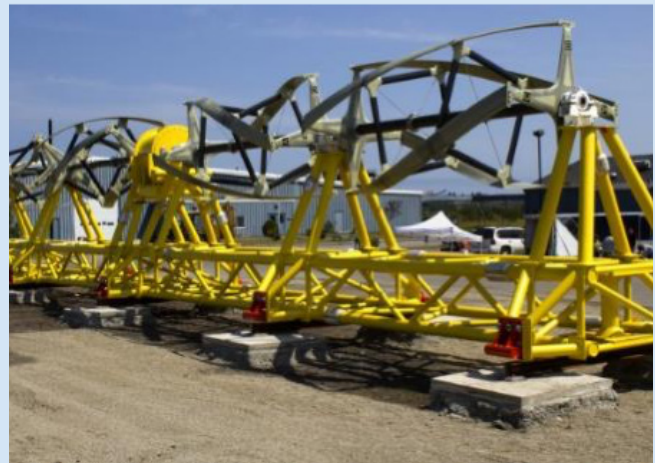
(Top and Middle) ORPC's Patented turbine generator units (TGU(s)) mounted on the TideGen delivery system, ready for shipment and deployment. Images Source: Ocean Renewable Power Company.
