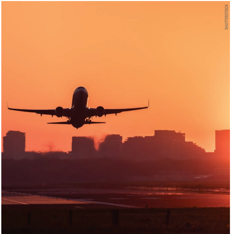
High temperatures decrease the density of air, making it more difficult for planes to achieve the lift necessary for takeoff. To compensate, airlines can decrease the cargo weight, but under future worst-case-scenario climate projections, planes may need more runway distance to achieve the necessary lift.
