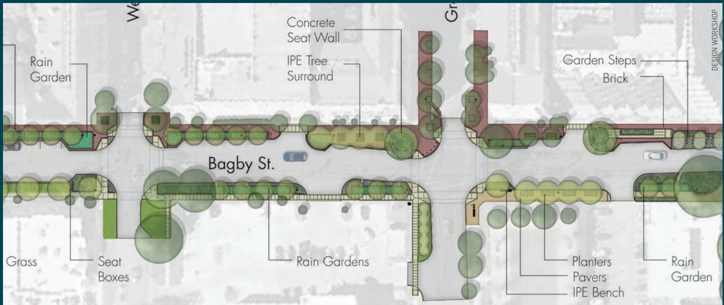
The master plan for Bagby Street added 175 new large shade trees to provide 90 percent shade coverage along the corridor, achieving a 20°F reduction in the shaded areas.
