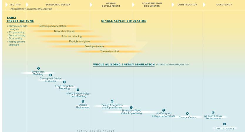
ASHRAE Standard 209 defines whole-building energy simulation in terms of 11 cycles that correspond to architectural design phases. Single-aspect simulations, performed or led by the architect, are important to inform the analyses performed in these cycles.
