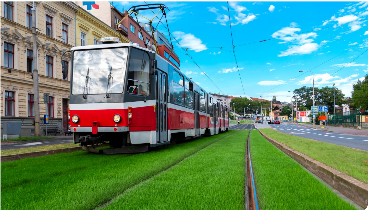
In many European cities, tram tracks are lined with grass, reducing the urban heat island effect and providing a permeable surface to aid in stormwater management.
