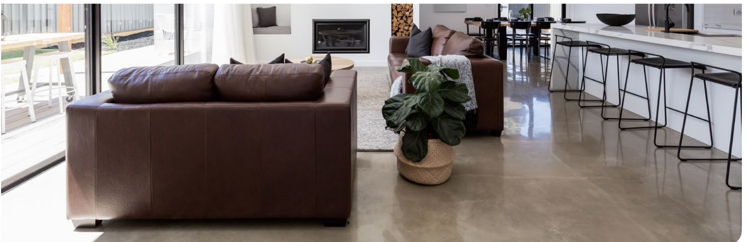
Water-resistant finishes like polished concrete floors are attractive and require little maintenance after a flood.
