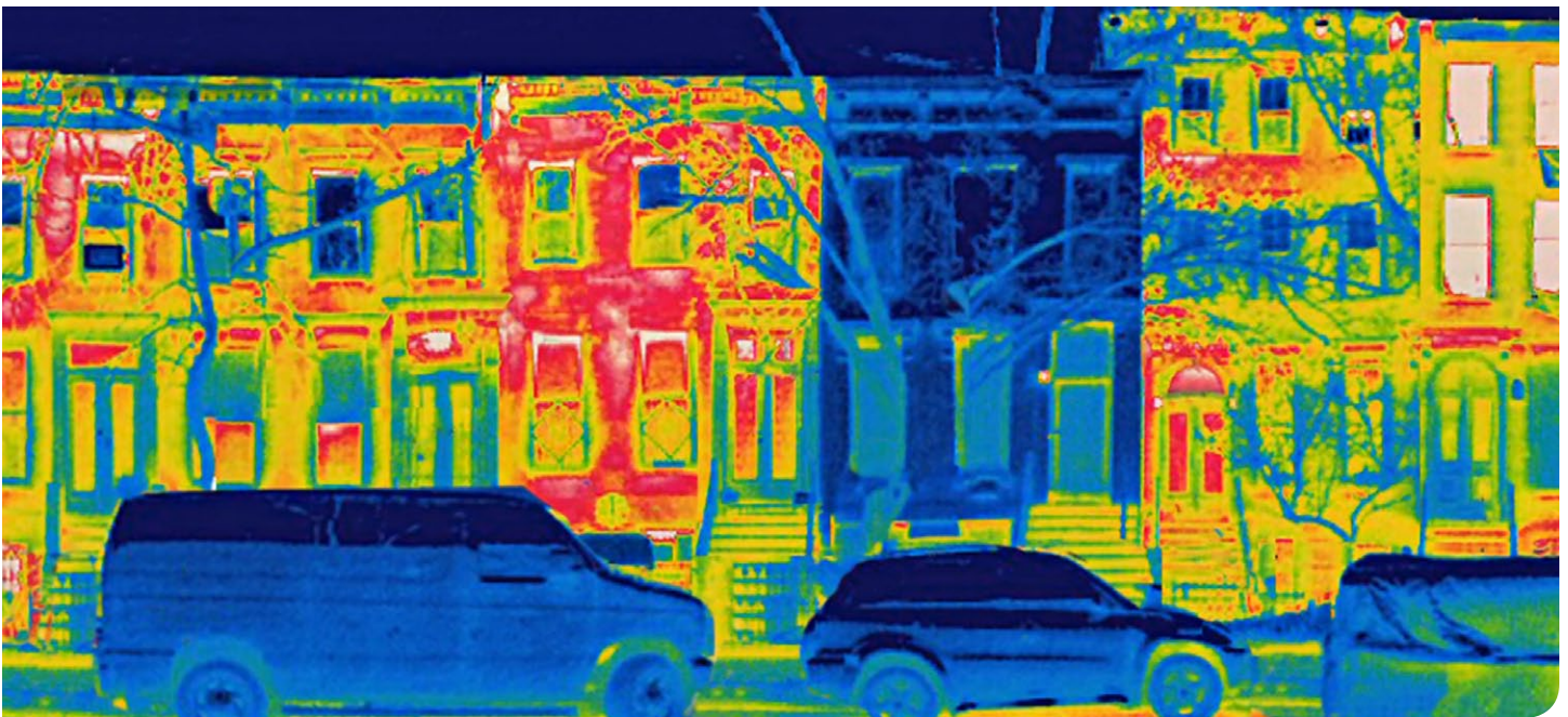
Passive House retrofits (building in blue) can drastically increase protection from extreme temperatures, keeping buildings comfortable in hot and cold weather.
