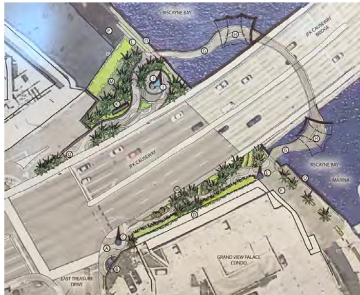
Preliminary Design for Waterfront Pedestrian Bridge under the Causeway to connect future sections of the Island Walk. Design by Kimley Horn.
