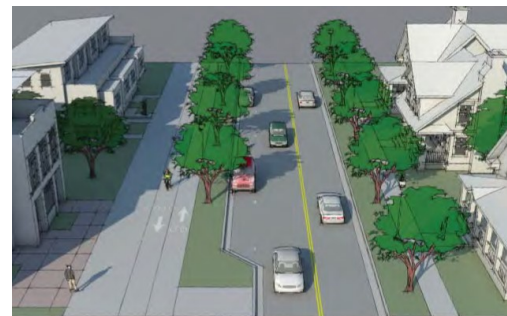
Proposed Colorado Boulevard section in STAMP with off-street bike lanes, on-street parking, and sidewalks on both sides. Rendering courtesy Commerce City Station Area Master Plan.
