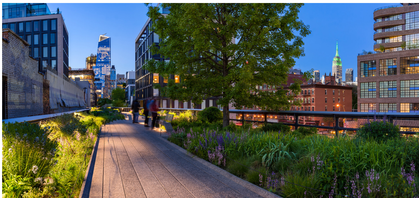
Examples of nature-based solutions for reducing the heat island effect, including tree canopy preservation, native vegetation lining walkways, and use of permeable surfaces for walking paths.
