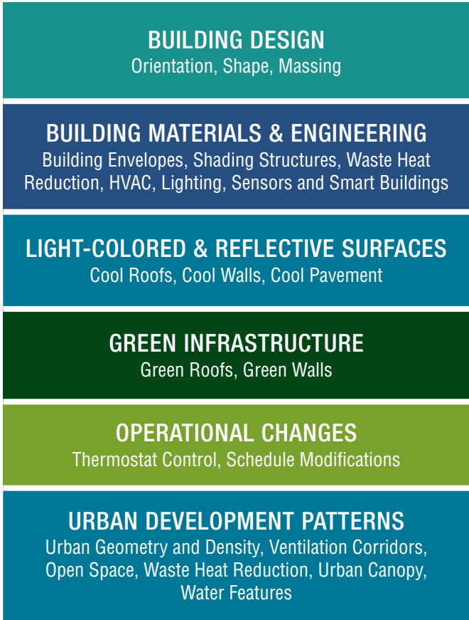
A potential heat resilience toolkit for developers might cover a range of building design, material, and urban planning aspects.
