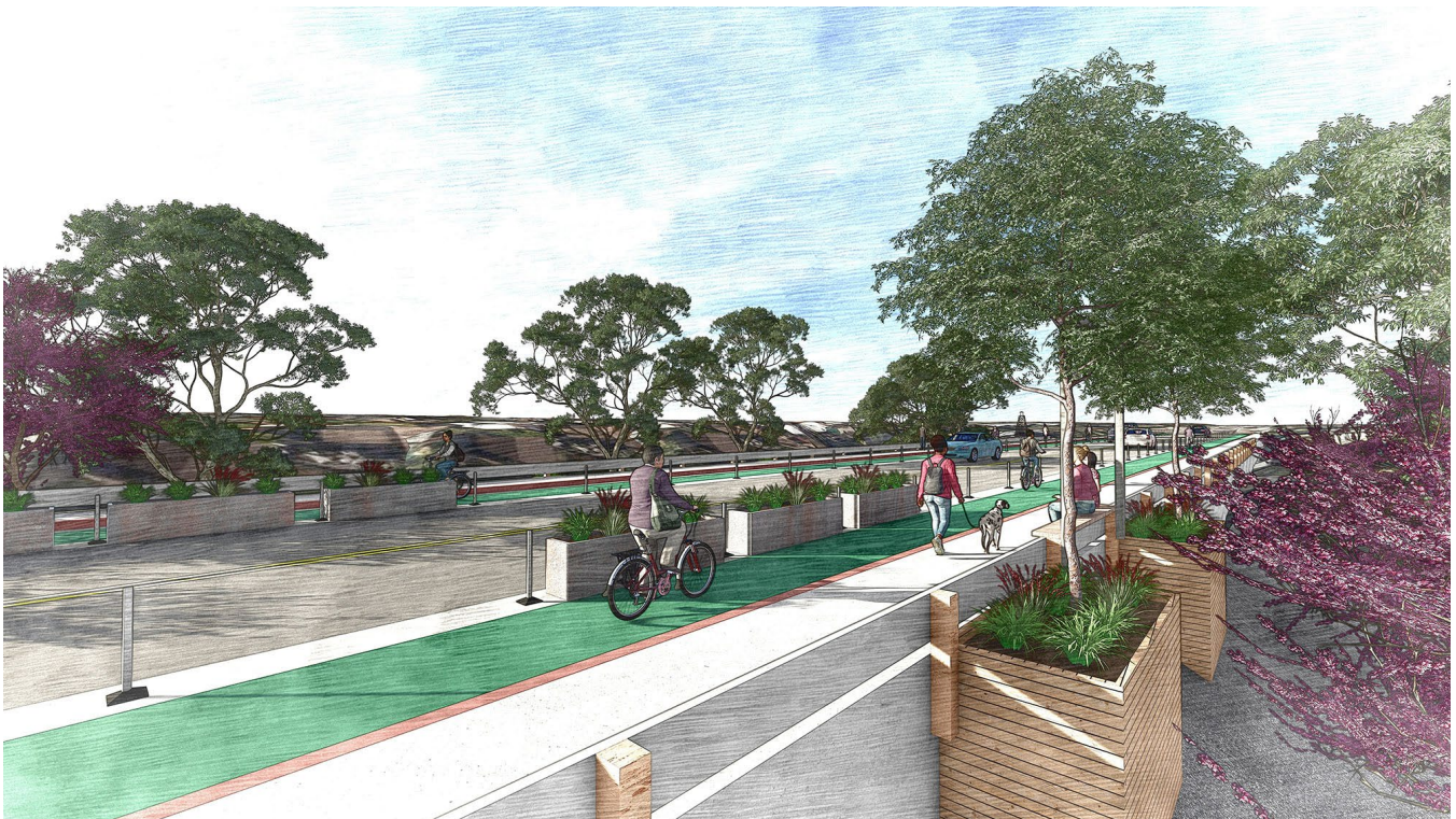
Trees can be planted at street level using planter boxes built behind, and anchored to, the guard rail; tree-lined streets have a traffic calming effect; pedestrians enjoy shade from street-level trees.
