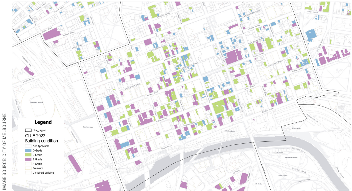
Figure 9: CLUE 2022 - Building condition by grade (B, C and D grade highlighted)
