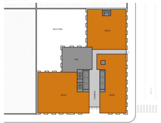
Diagrammatic site plan for ground floor from Downtown SF office-to-residential repositioning study completed by SPUR; Gensler. G
