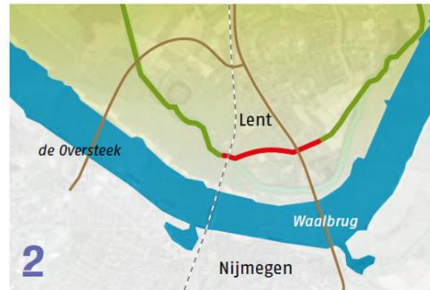
The dike was moved 350 metres inland.
